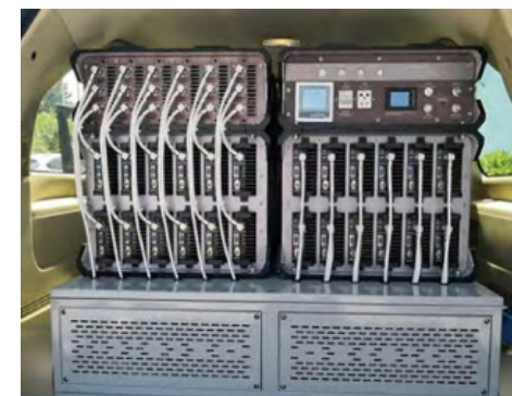
1300 Watts 24 Bands 20-6000MHZ Vehicular Jamming System for military VIP convoy protection
